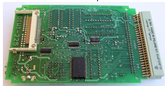
DivIDE Plus board: bottom side with CF card slot
